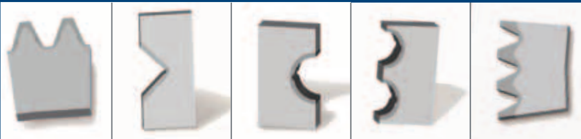
Tempra dente per dente Tooth by tooth induction hardening
